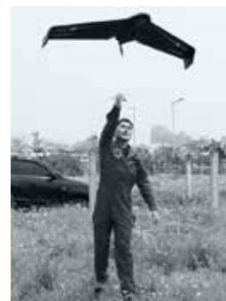
Pterosaur™, an ultralight drone created by GEOSAT, features fixed wings like a stealth aircraft. One might think that it would be difficult to operate, but according to the developer, basic operations can be mastered in only ten minutes. Its landing mechanism, which mitigates shock by deploying a parachute to flip over the drone, is popular among professionals. → p. 62
