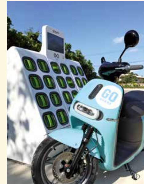
A Go Station, where used batteries can be exchanged with ease.
