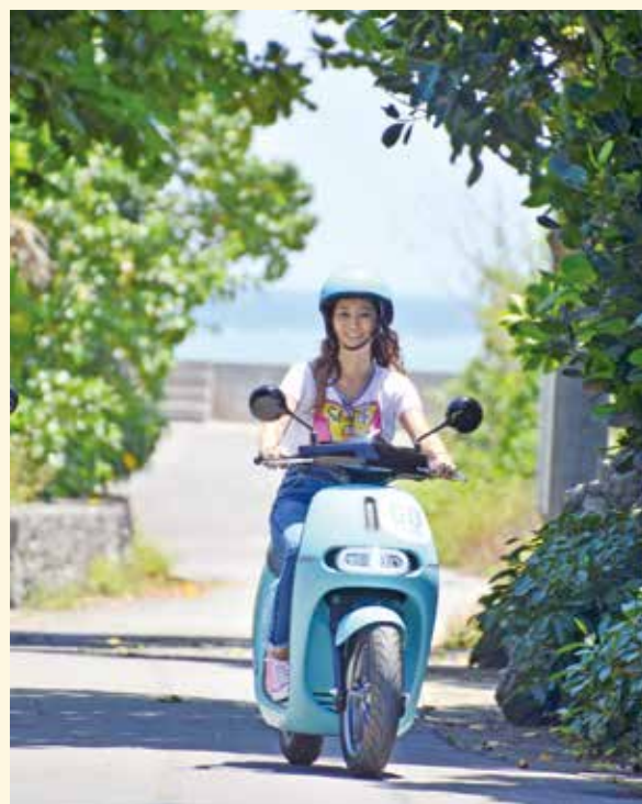
An electric scooter with a replaceable battery made by Gogoro, Inc. Battery replacement can be performed at unmanned battery stations called Go Stations, and takes just a few seconds.
